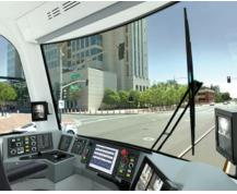
Each streetcar is electrically powered from an overhead catenary system (OCS) and for Orange County operates at speeds up to 44 mph, carrying close to 220 passengers in each vehicle. These streetcars remove automobiles off the road, in turn helping cities decrease their CO2 emissions.
